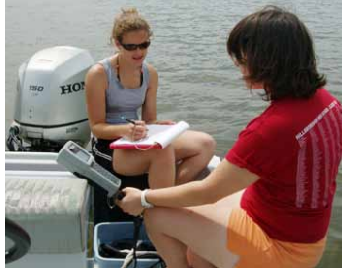
Interns measure dissolved oxygen concentrations in the Chesapeake Bay. Water is typically considered hypoxic if oxygen concentrations are below 2mg/L. Photo: Courtney Richmond
