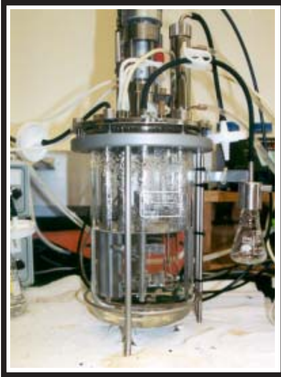
Figure 2. One of the bioreactors used to test the influence bacteria on Fe oxidation.
