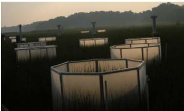
*Experimental chambers are used to raise the amount of CO<sub>2</sub> in the atmosphere of a tidal wetland plant community.*
